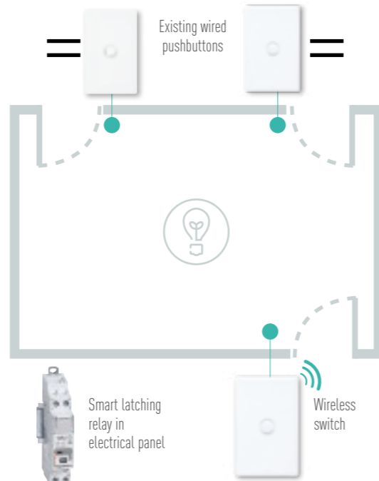
REFURBISHMENT INSTALLATION (replacing a latching relay)
